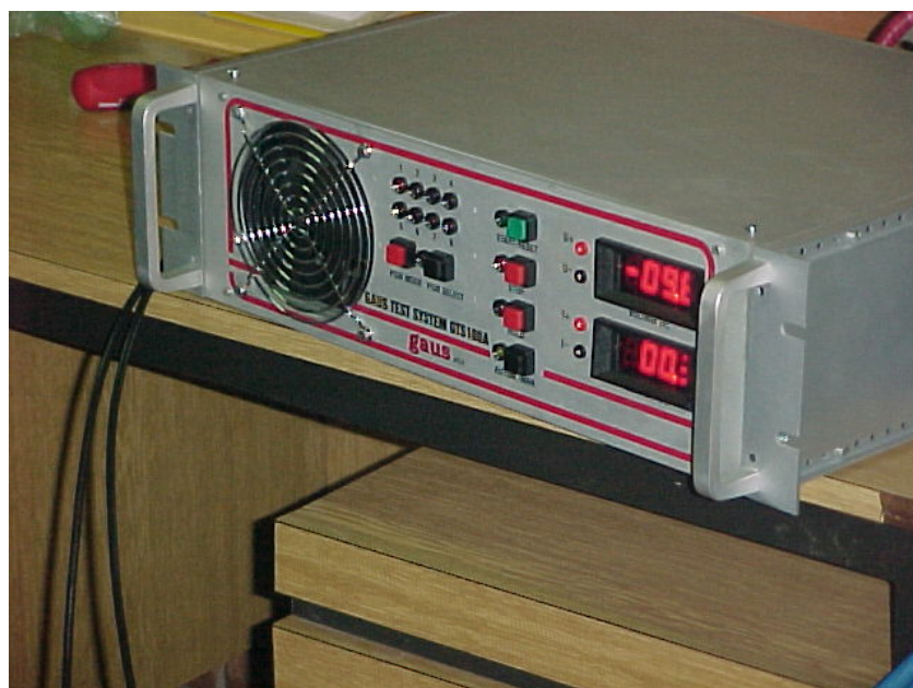
Figure 1. Device for measuring transitional resistance between contacts of disconnectors, switch disconnectors and circuit breakers in transformer stations
